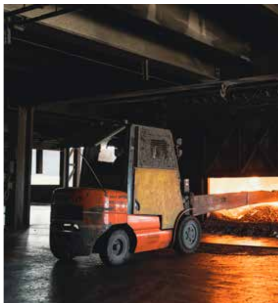
The furnace is being fed with raw materials
